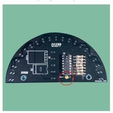
Step 4: Place and solder the **Humidity Sensor** into place.
